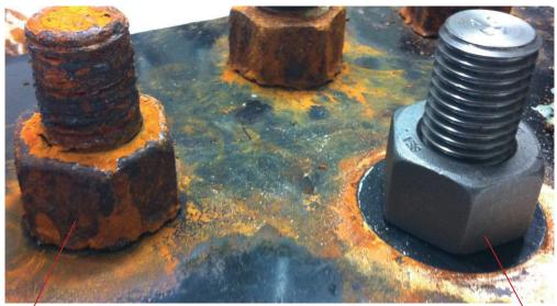
ASTM A193 B7 1" STUD BOLT & gr 2H NUT EXPOSED TO SALT FOG FOR 600 HOURS
