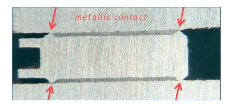
The soft layers function is primarily to act as a limiter and to clearly regulate the max. load to be applied on to the gasket.
