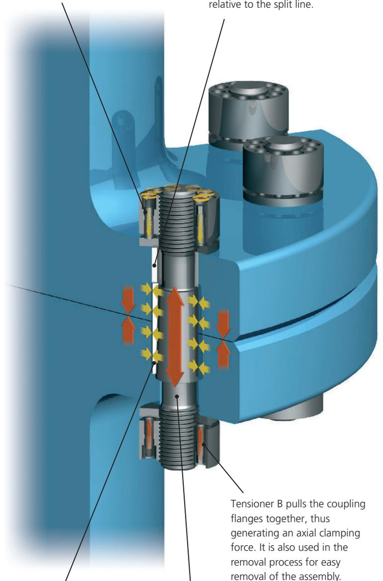
The split tapered sleeve creates a radial pre-load and transfers the external torque.
