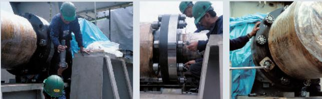
Superbolt Expansion Bolts are used to tighten the flange connections on ship propeller shafts, which otherwise requires the coupling holes of the flange to be fitted accurately and machined on location when mounting the fitted bolts. The Expansion Bolts were tightened easily and quickly with only standard tools.
